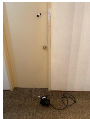
Figure 6: Air sampling monitor cassette & pump used for dust recording
